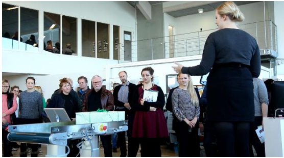
Figure 9 - The MiR robot with the conveyer belt on top is demonstrating automatic transportation of boxes
